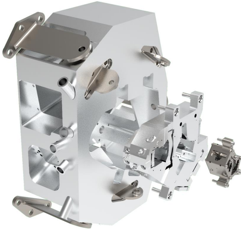
Figure 7 Rendering of the SPEXone opto-mechanical housing and its nested build-up showing from large to small: the spectrometer, the telescope and the PMO. Overall size 10 x 20 x 30 cm 3 .
