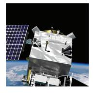
The central part of PACE is called a "bus." It serves as the hub for the spacecraft, providing places to mount science instruments, solar array, communications equipment, etc. It also houses electronic systems that distribute power and information needed to operate the spacecraft.
